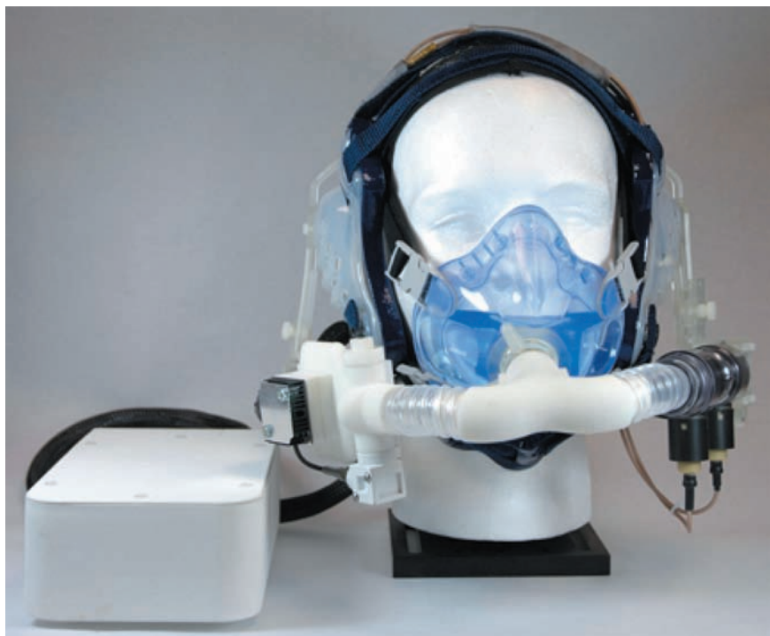
Figure 8.1 A portable device to measure oxygen consumption and carbon dioxide production. The headgear contains oxygen and carbon dioxide sensors on the left side and the flow sensor on the right side, all tethered to an electronics box (to the left of the headgear) that fits into a small wearable pack.
