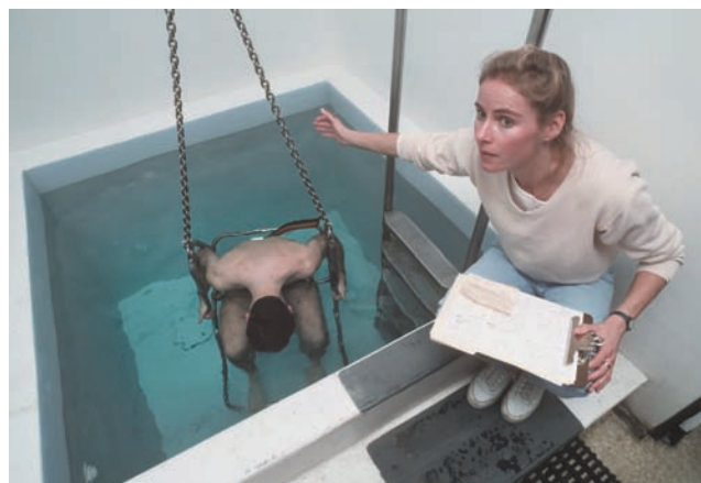
Figure 8.9 Apparatus for underwater weighing to determine body density.
