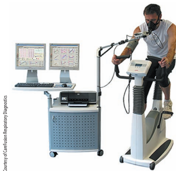
Figure 8.2 A metabolic cart (shown here with bicycle ergometer) measures oxygen consumption and carbon dioxide exhaled.
